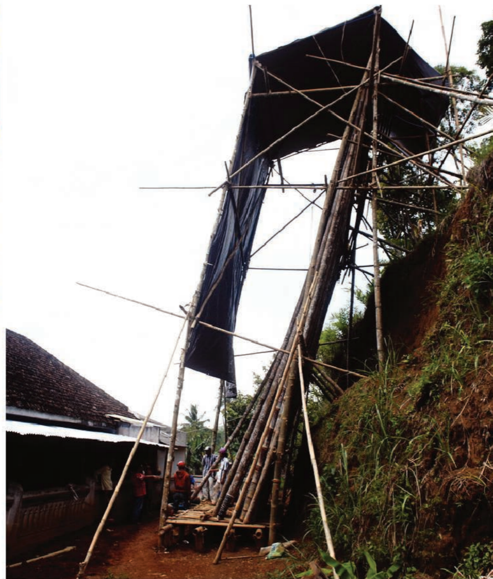
Treatment tower to provide durable bamboo poles for permanent use in construction ▶
